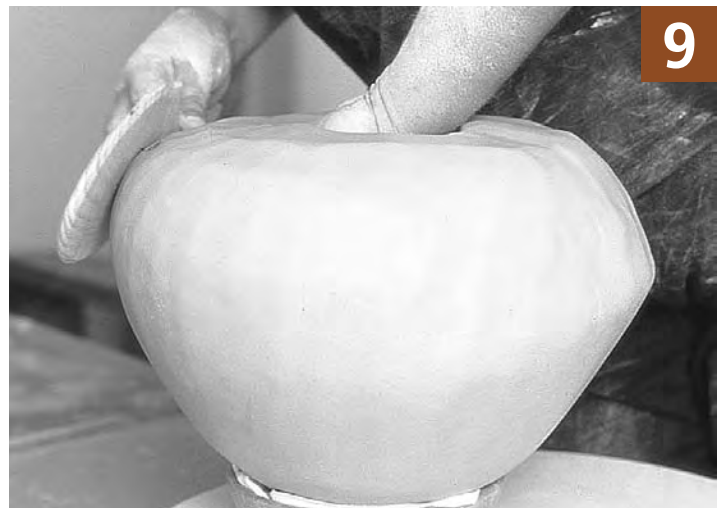
Subsequent passes refine the curve of the shoulder; eventually, the paddle is used simply to control the amount of stretching.
