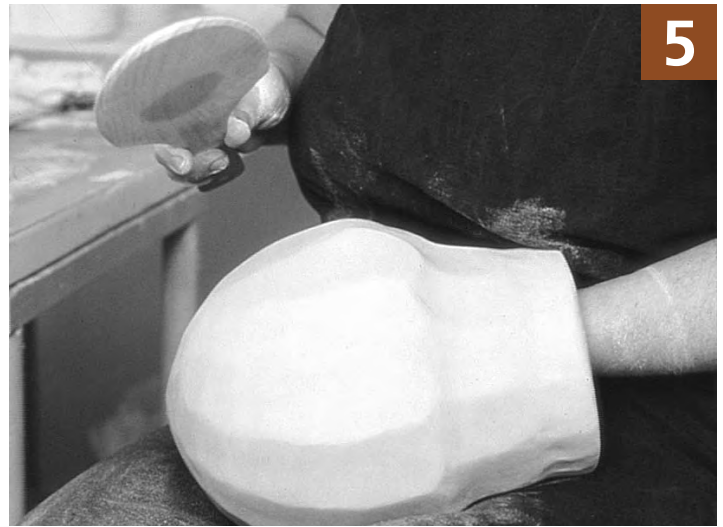
After the clay has hardened somewhat, the lower wall is stretched more, reserving a small amount of clay at the bottom.
