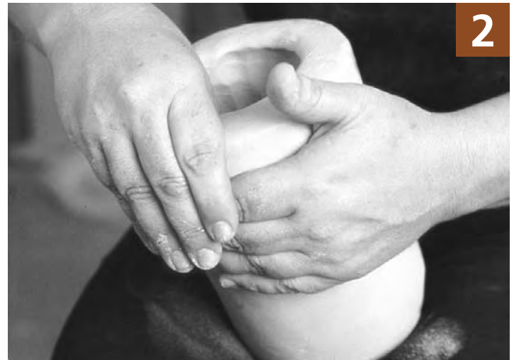
The upper walls are thinned by pushing with the thumb from the inside, while supporting the outside with the outer hand.
