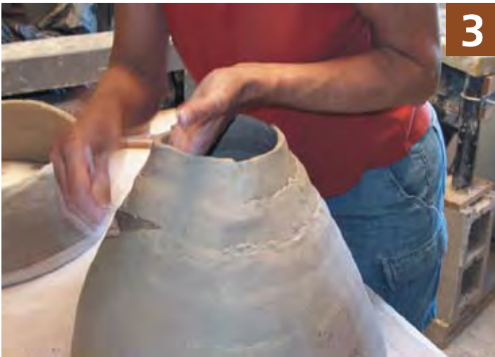
3 Smooth the seams inside and out.
