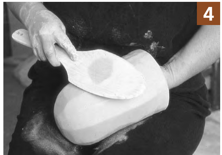
The wall thickness is evened (bottom to rim) by rhythmical paddling while slowly rotating the form with the inside hand.
