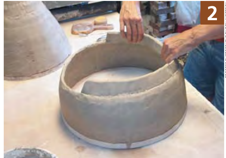
2 Build the lower section upside down.
