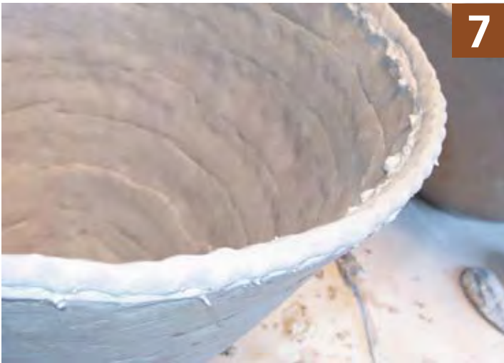
Flip the form over and add a coil.
